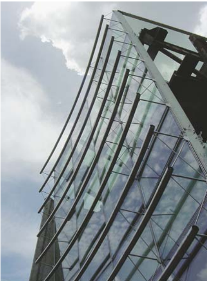
Beacon Court curtain wall visual and performance mock-up
