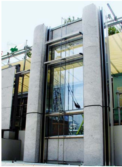
Curtain wall visual and performance mock-up
