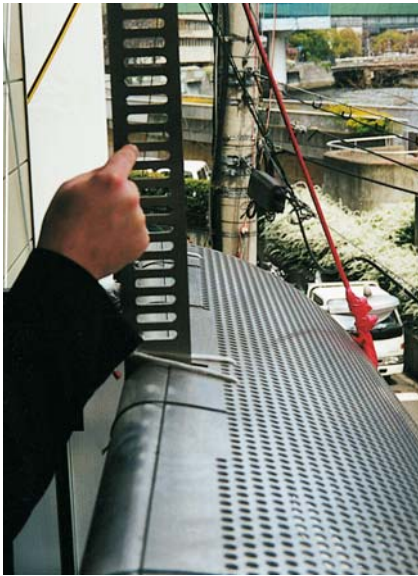
Perforated sunshade corrosion performance test
