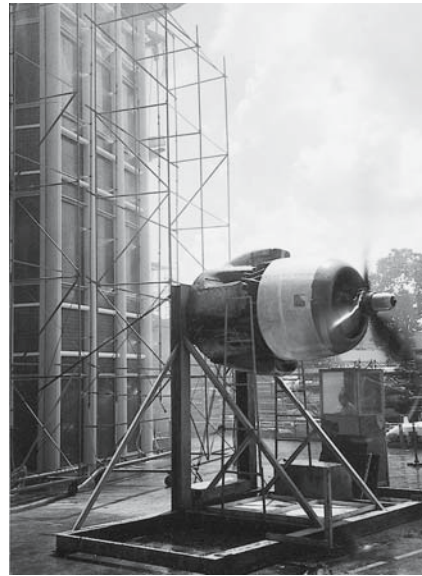
Curtain wall performance mock-up, International Finance Centre
